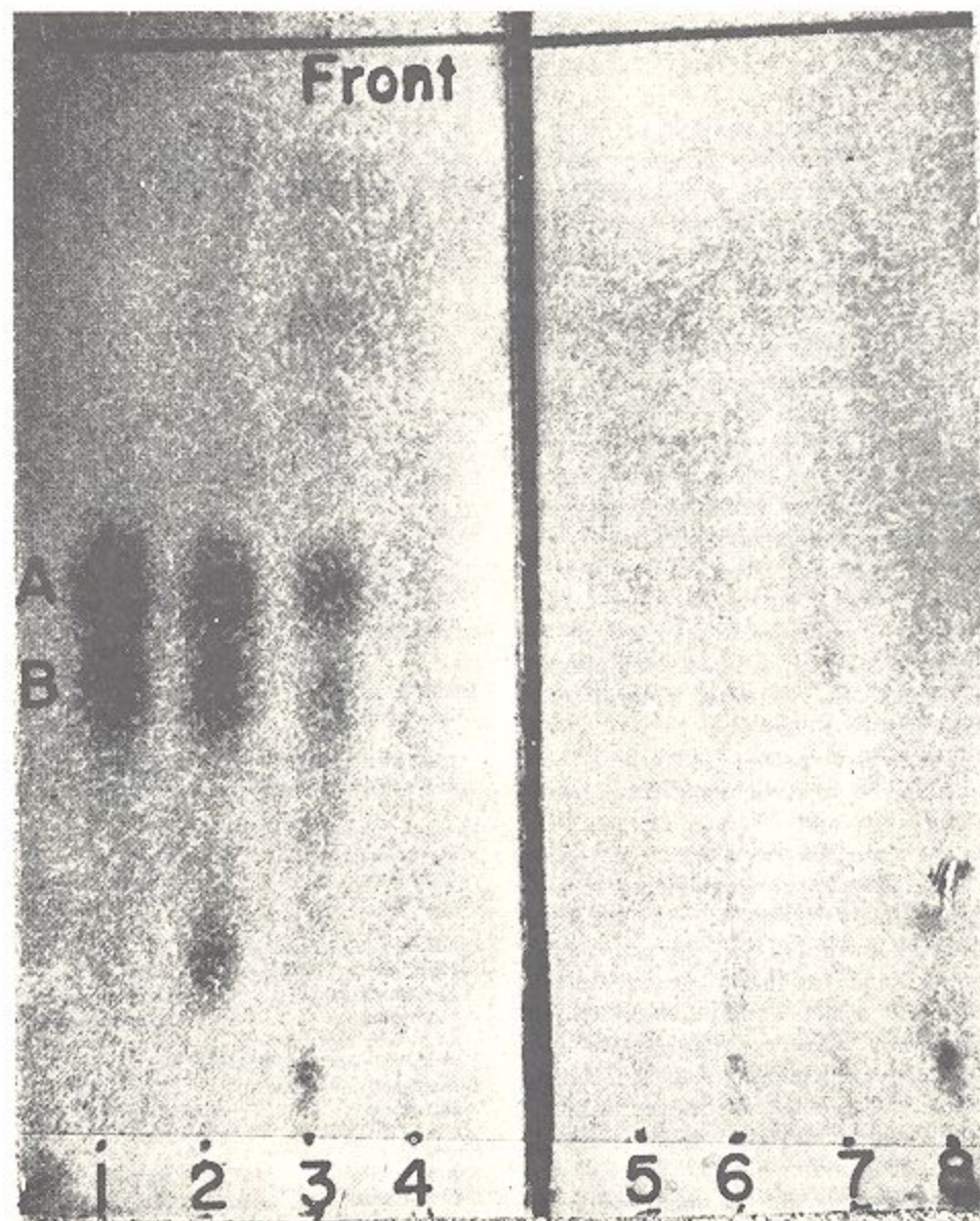
Fig. 2. Thin-layer chromatography (silica gel-G; solvent was a mixture of 50 parts methanol, 5 parts chloroform, and 0.5 part 6N ammonium hydroxide; detection with iodine vapor) of compounds A and B in partially purified skin extracts from samples of Dendrobates pumilio . The sample designations (1-8) correspond in order with the populations listed in Table 2. Concentrated samples with the equivalent of 5 mg of skin were chromatographed.
